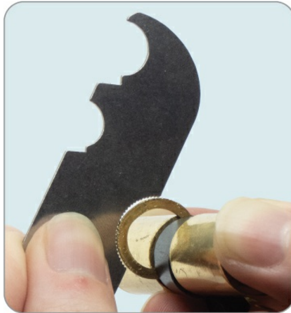
Figure 5-26: Reinstalling a C-clip using the SPARROWS Gut Wrench
