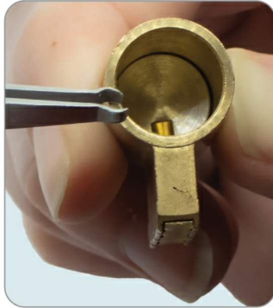
Figure 5-22: Installing a driver pin in the bible
