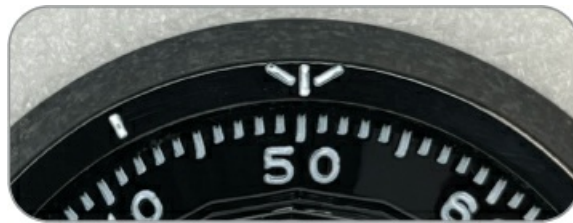
Figure 14-2: If any portion of the number index line is under the opening index, it counts as an overlap, so this is 50 Overlap.
