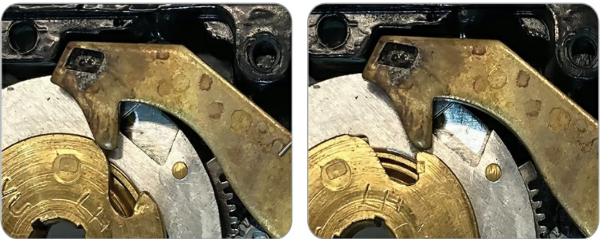
Figure 13-3: Left: The right contact point as seen from the back of the lock. You dialed left to get to the right contact point, which is on the right side of the dial when facing the lock. Right: The left contact point as seen from the back of the lock.
