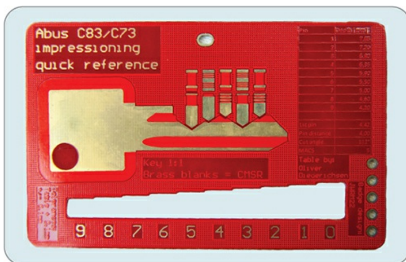
Figure 9-20: A key gauge integrated in a LockCon conference badge (excellently designed by Jan-Willem Markus)
