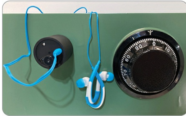
Figure 12-5: This old filing cabinet drawer has been turned into a dialing station—not particularly handy to carry around, but the EZ AMP attaches to this solid metal surface magnetically.
