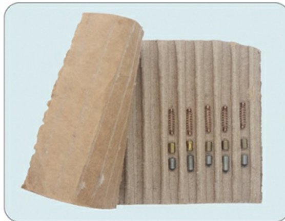
Figure 5-5: Corrugated cardboard: the world's most readily available pinning tray
