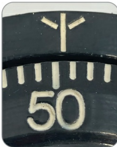
Figure 13-4: A reading of 50.4 or 50.5
