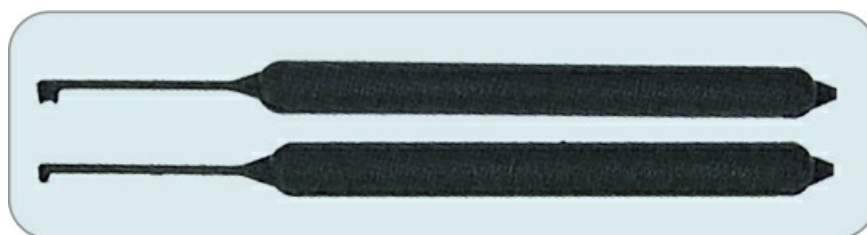
Figure 6-16: Dimple picks for a pin-in-pin Mul-T-Lock; the top pick is for the outer pins, and the bottom is for the inner pins
