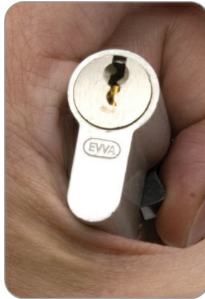
Figure 7-6: Tensioning the cam on a Euro profile cylinder
