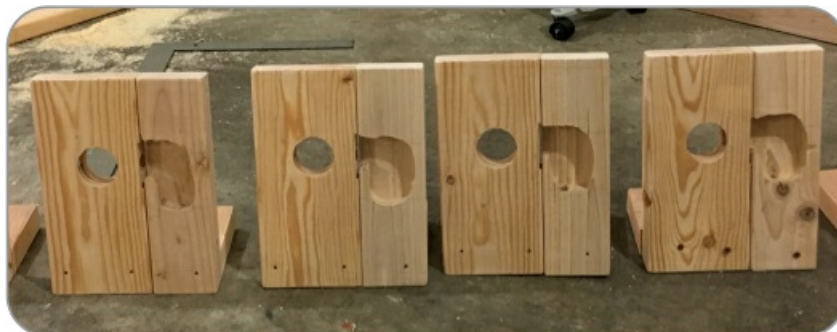
Figure A-4: A batch of stands with holes drilled for the locks, and pockets cut for the bolts and switches
