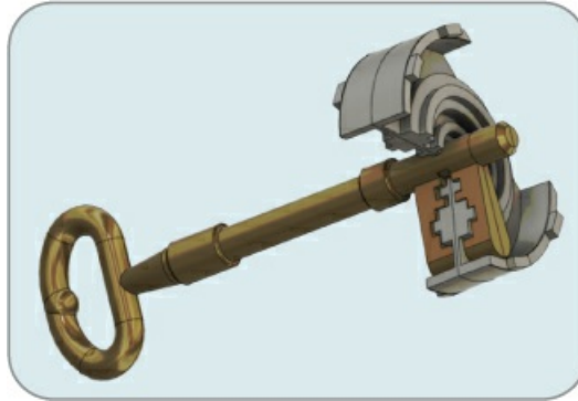
Figure 3-31: A warded lock and its key
