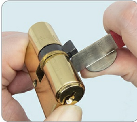
Figure 5-12: Prying a C-clip loose with a clip remover
