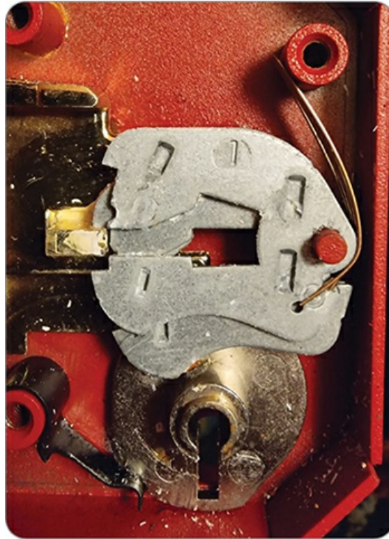
Figure 16-1: The topmost lever in this UNION StrongBOLT is in the true gate, while the levers behind are as yet undisturbed.
