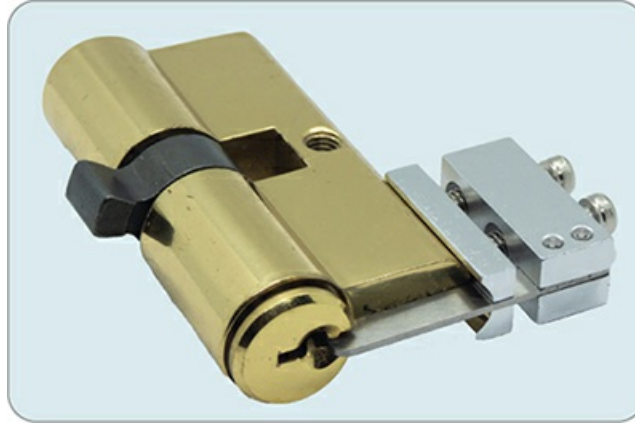
Figure 5-14: A double-sided Euro profile cylinder with a pinning shoe inserted to retain the driver pins
