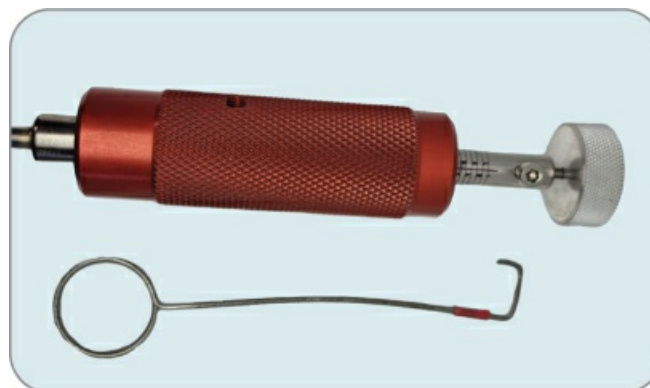
Figure 15-23: Both of these tools started off straight: the handle to a custom-made pick for the Mauer 71111 President lock, complete with engraved spacing markings for each lever, by Jason Jones at https://www.kelocks.co.uk (top), and a J wire (bottom).
