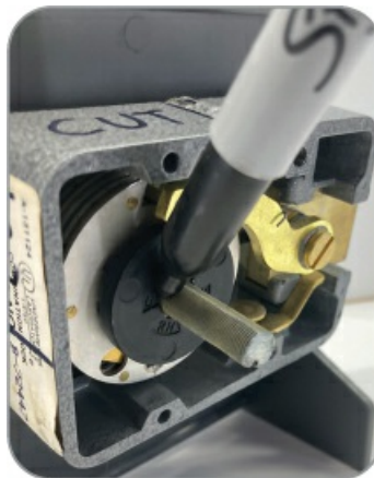
Figure 12-6: If you have to mount and cut your spindle to size, assemble the lock first to mark the fit.
