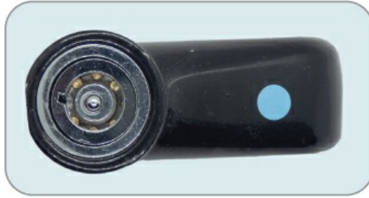
Figure 3-24: A tubular lock with seven pins
