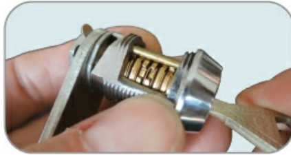
Figure 7-28: A cutaway ASSA ABLOY Classic lock
