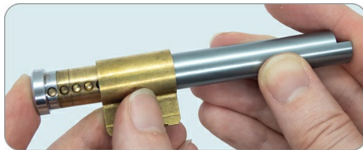
Figure 5-16: A plug follower pushing a plug out of its housing
