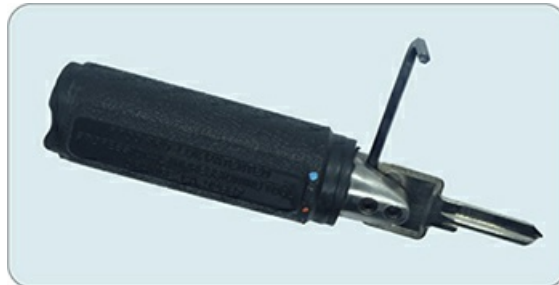
Figure 9-2: A Pro-Lok handle with an Allen wrench as a lever
