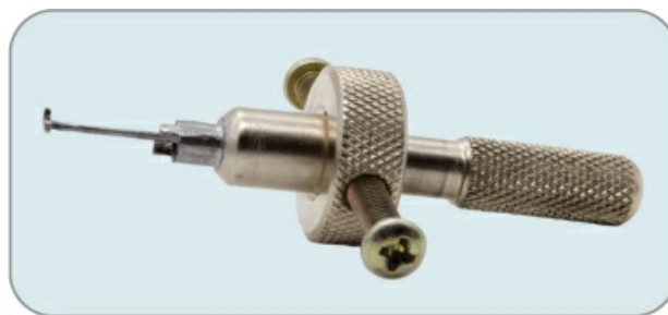
Figure 7-33: Homemade tool to pick a DOM Diamant
