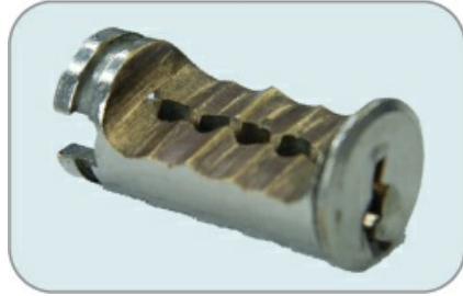
Figure 10-35: A filed-down ABUS plug
