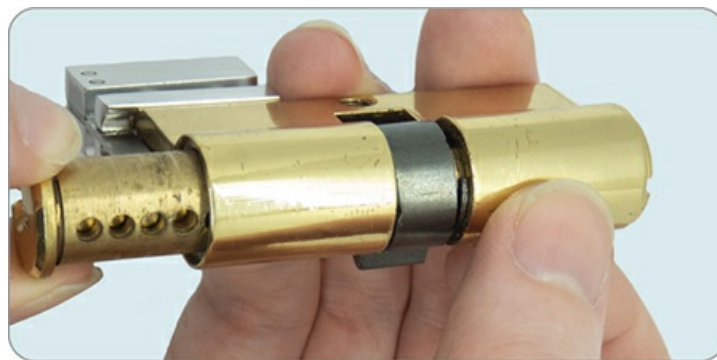
Figure 5-15: Top-down photo of pulling a plug from one side of a Euro profile cylinder
