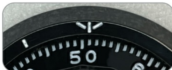
Figure 14-7: The opening index is centered on the next number, and the process starts again. This is 51.
