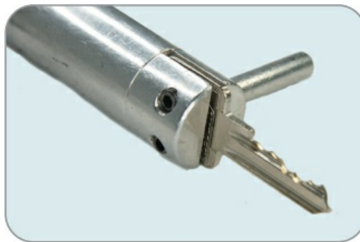
Figure 9-5: A KJS Tools impressioning handle with lever, custom-made by Jord Knaap
