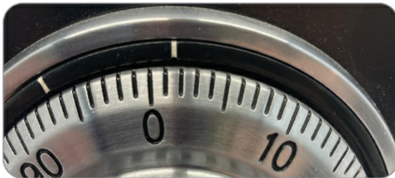
Figure 13-11: The left contact point is reading around 1.5 with no gate under the fence.
