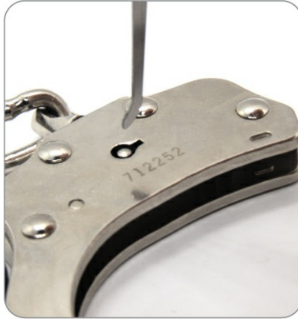
Figure A-14: Proper orientation for the picking tool to open handcuffs
