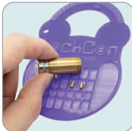
Figure 5-18: Dumping the key pins from the plug
