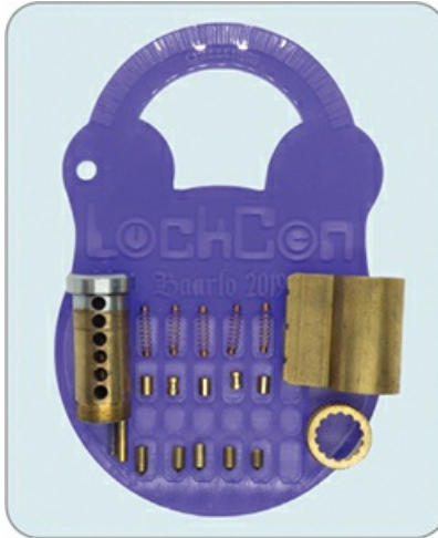
Figure 5-4: A laser-etched pinning tray holding a disassembled KIK cylinder
