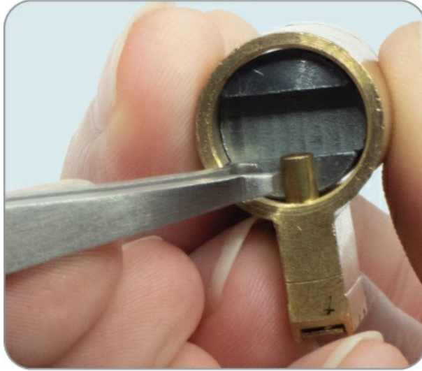
Figure 5-19: Releasing a driver pin
