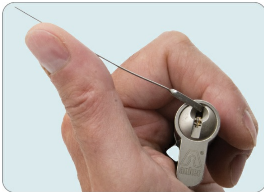
Figure 7-2: Another way of holding a cylinder and tension wrench
