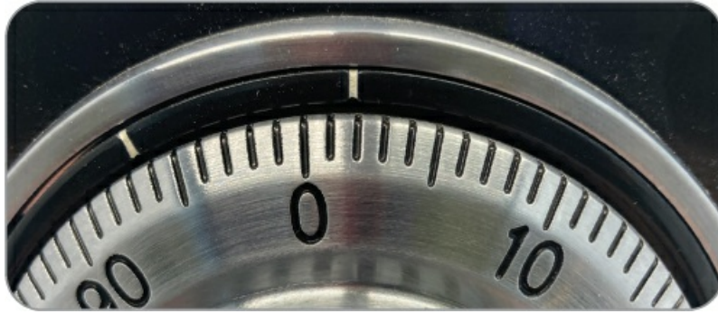
Figure 13-12: Notice that the reading has shifted slightly right when the fence slips into the gate.
