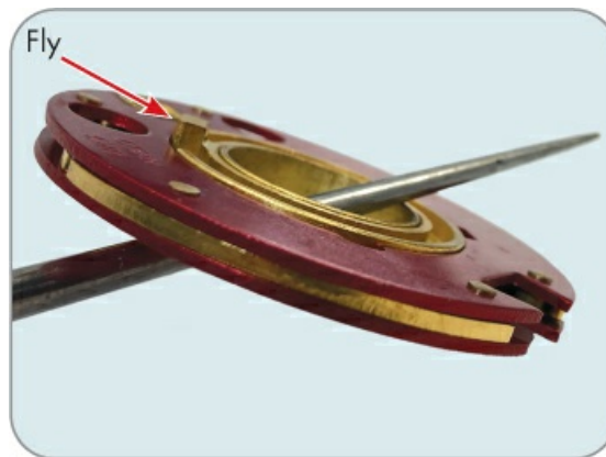
Figure 12-17: Wheel 3, the one closest to the drive cam, always has a protruding fly, while all the other flies are flush with the wheel.
