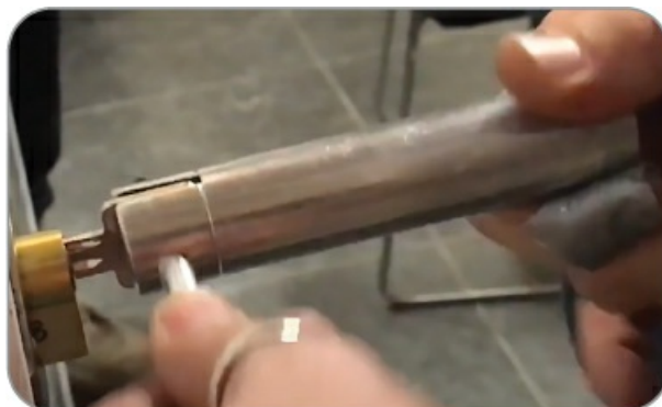
Figure 10-9: The double-handed jiggle technique: the nondominant hand does all the turning, while the other does all the jiggling
