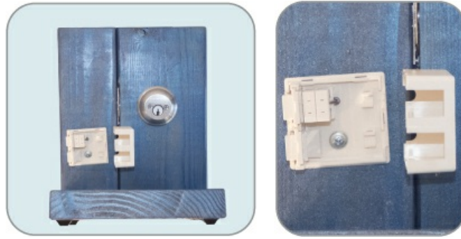
Figure A-6: The back side of a completed stand with an open keystone box (left) and a close-up of wires feeding into the RJ45 jack
