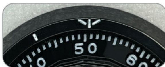
Figure 14-5: The opening index's right side is starting to align with 51's left side, so this is 50 Next Aligned.
