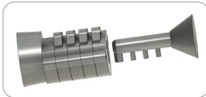
Figure A-20: The wheels of a direct-entry combination lock (left) and the shackle (right)
