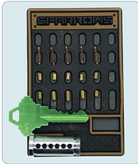
Figure 5-20: A pinning tray with key and driver pins selected to match a key
