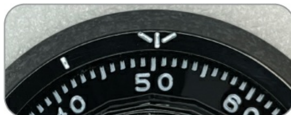
Figure 14-3: Because the edges of the opening and number index align, this reading is considered 50 Aligned.
