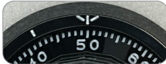
Figure 14-1: A perfectly aligned reading of 50
