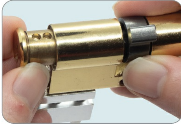
Figure 5-25: Reinserting a plug and cam into a Euro profile cylinder
