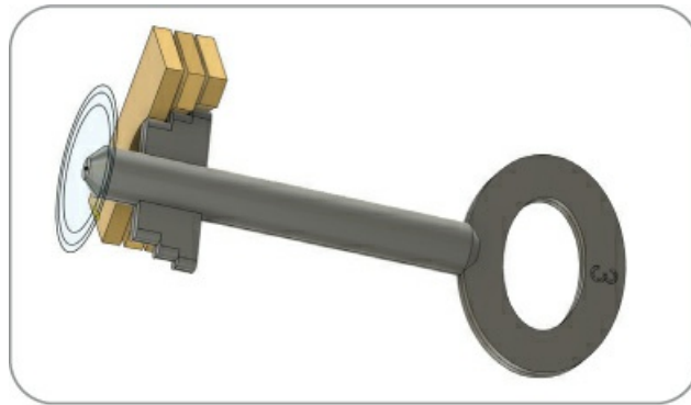
Figure 16-5: This lock couldn't have near-identical bellies unless the gates were curved, but regardless, simply lifting the toe or heel of all the levers together, perhaps with a J wire, would open it!
