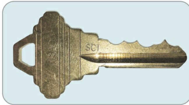
Figure 10-34: A successfully impressed Schlage key
